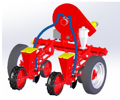
Fig. 1. Seed drill equipped with cyclone for dust collection
